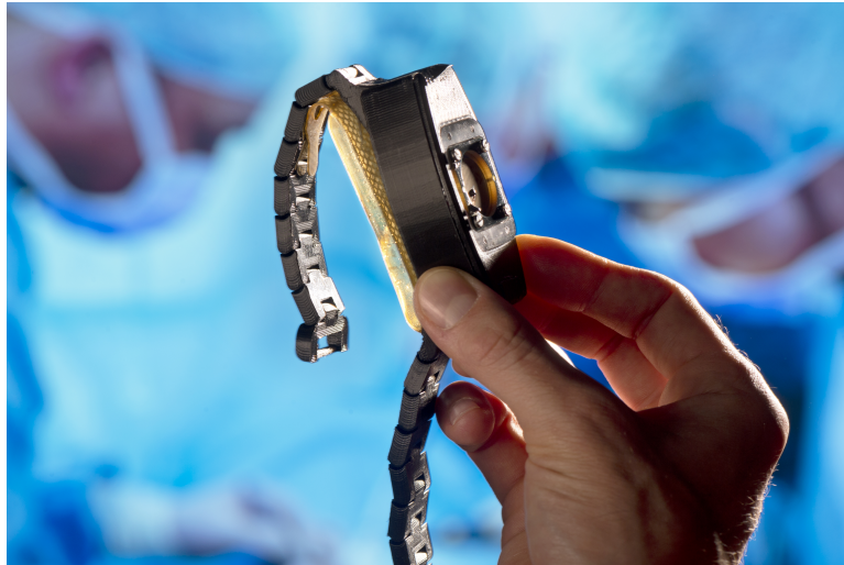
Figure 4.2 Implementation of a wearable blood pressure measurement prototype with an integrated micropump. The cuff is visible in yellow at the lower side of the wrist holder © [137].
