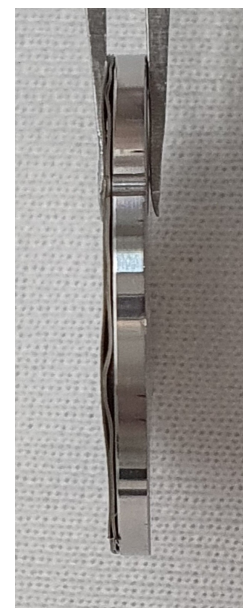
(b) Specimen with a corrugated foil stack due to a strong and direct heat impact during laser-welding.
