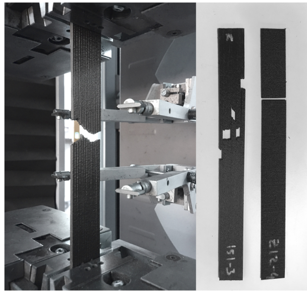
Figure A1. Longitudinal test specimen after failure in the universal testing machine and representative test specimens in x (left) and z (right) directions after testing.
