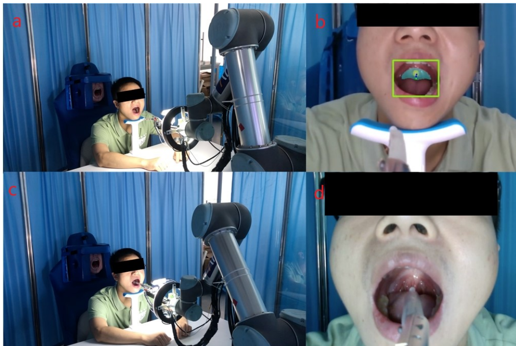
Figure 2.11: Sampling process from vision detection to sampling tasks. In our experiments, many volunteers were tested, and the recognition rate, control precision, sampling time, and sampling contact force were recorded.
