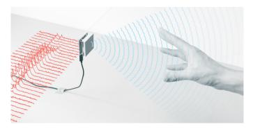
Figure 6.1: Radar-based hand gesture recognition. (Figure from [231])
