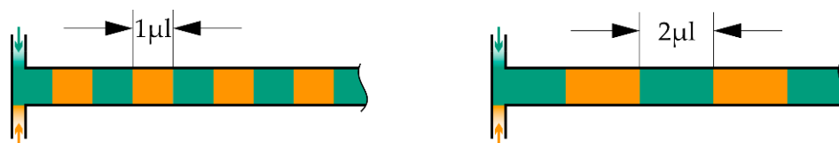
Figure 5. Visualization of different fluid packet sizes inside the microchannel. Of course, the zebra stripe pattern is for illustration purposes only and will not be present in reality due to mixing effects and diffusional transport.
