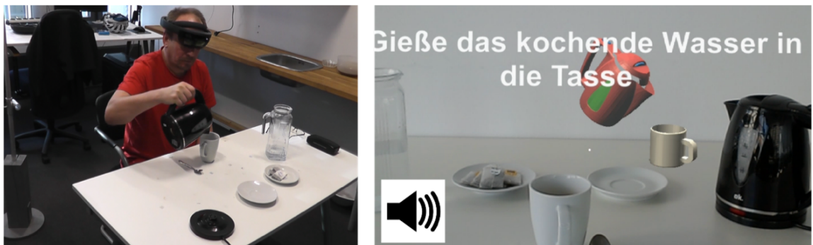
Figure 5. Experimental setup in study II. A patient is preparing a cup of tea supported by multidimensional cues delivered through the HoloLens glasses; i.e., animated holographic objects, text and audio information that direct the next step (Rohrbach, Gulde, et al., 2019). The participant provided consent for the use of the image. (Copyright left picture: Nina Rohrbach / TUM).
