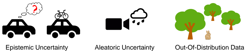
Figure 2.7 There are three main sources of failures in autonomous driving. Epistemic uncertainty stems from an insufficient model. Aleatoric uncertainty is inherent to the input. Finally, Out-of-Distribution (OOD) data differs significantly from the training set distribution.
