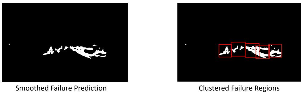
Figure 5.5 Visualization of the clusters obtained from the smoothed failure prediction using the k-means algorithm. Each cluster is shown via a red bounding box around the pixels belonging to the respective cluster.
