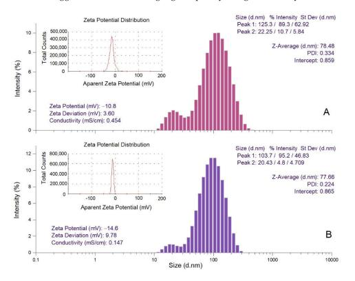
**Figure 5.** DLS analysis of *Picea abies* (**A**) and *Pinus nigra* (**B**) bark extract derived AgNPs (Z-average—hydrodynamic diameter; PDI—polydispersity index; d.nm—diameter in nm).
