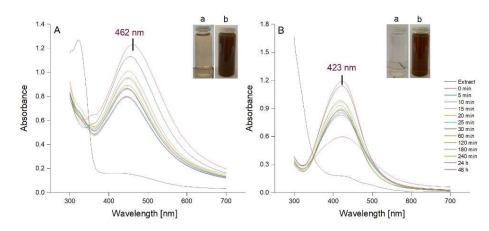
**Figure 2.** UV-Vis absorption spectra of AgNPs colloidal solutions synthesized using *Picea abies* (**A**) and *Pinus nigra* (**B**) aqueous bark extracts (a: extract + 1 mM AgNO<sub>3</sub> at time 0; b: extract + 1 mM AgNO<sub>3</sub> at 60 min).
