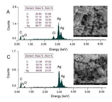
**Figure 6.** Elemental composition (EDX analysis) and scanning electron microscopy (SEM) micrographs of *Picea abies* (**A**,**B**) and *Pinus nigra* (**C**,**D**) bark extract derived AgNPs.
