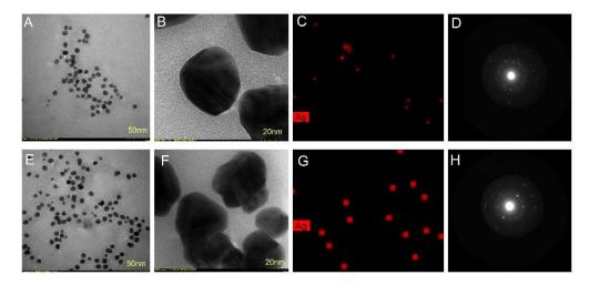
**Figure 7.** *Picea abies* bark extract derived AgNPs: TEM micrographs (**A**,**B**), TEM-EDX mapping (**C**) and SAED pattern (**D**); *Pinus nigra* bark extract derived AgNPs: TEM micrographs (**E**,**F**), TEM-EDX mapping (**G**) and SAED pattern (**H**).
