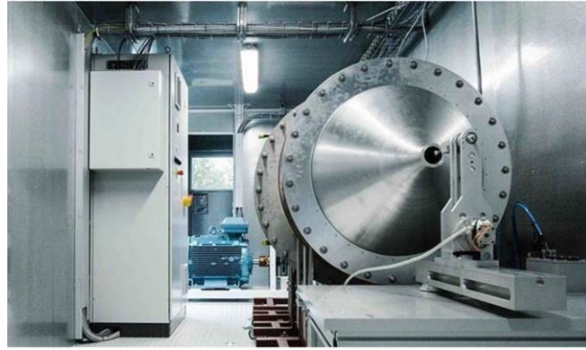
Figure 7. Free-jet calibration facility at Vectroflow [22].
