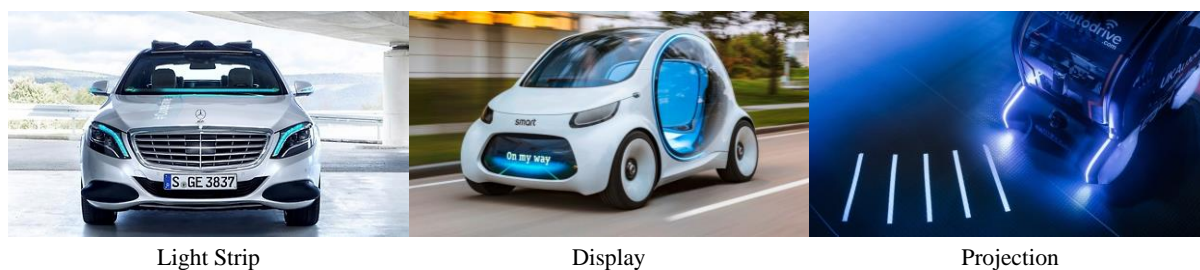
Figure 8: Different visual eHMI types categorized in the subgroups light-strip (Daimler AG, 2019), display (Daimler AG, 2017), and projection (Donath, 2019).
