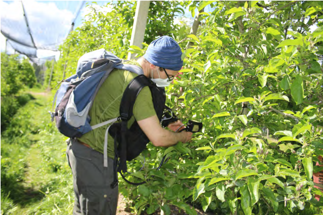
Figure 4.5: Leaf spectra Sampling using the hand-held spectroradiometer on the orchard
