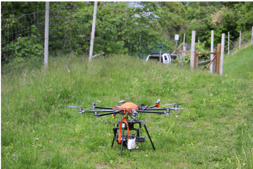
Figure 4.8: Soleon Octocopter mounted with the MicaSense Red Edge and the Rikola hyper-spectral camera
