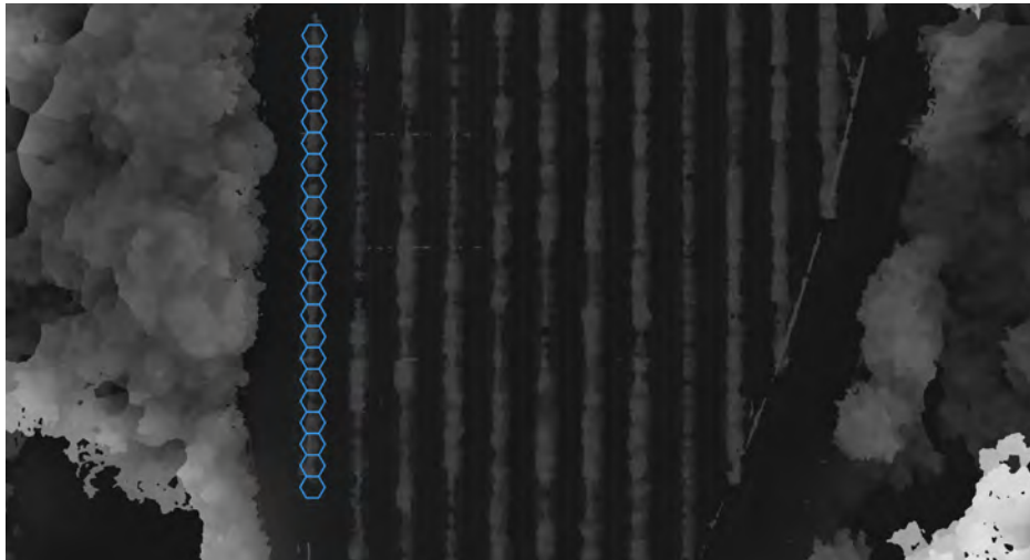
(b) Exemplary hexagonal grid structure for one tree row laid over the CHM
