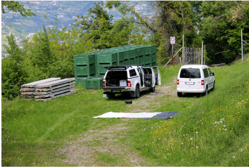
Figure 4.12: White, grey and black tarps used in the field for calibrating the Rikola camera
