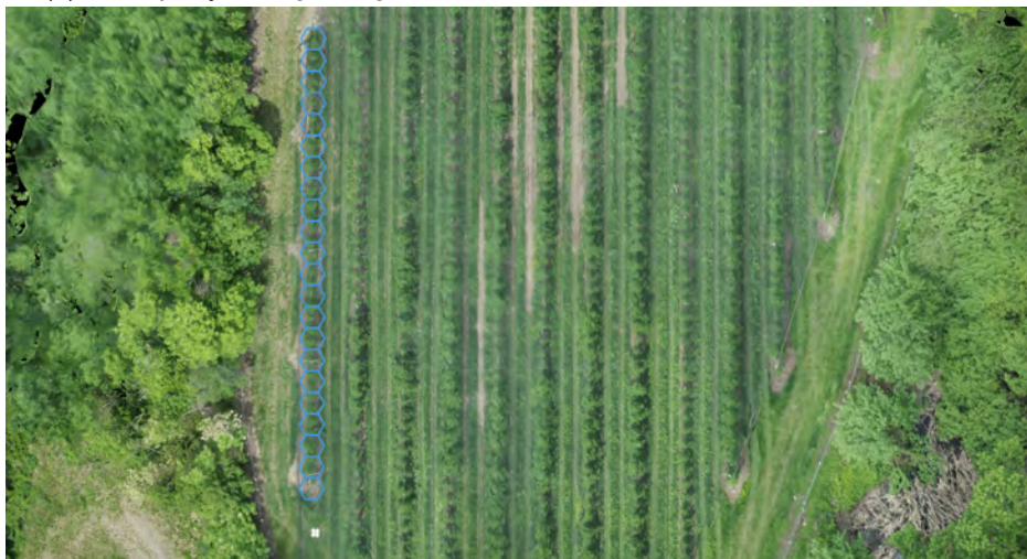
(c) Exemplary hexagonal grid structure for one tree row laid over the orthophoto
