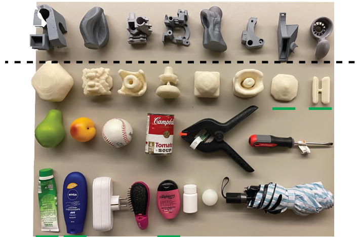
Figure 4.10: 32 physical objects for the grasp planning experiments. The objects with a green underline are flat objects, which are potentially difficult to grasp.
