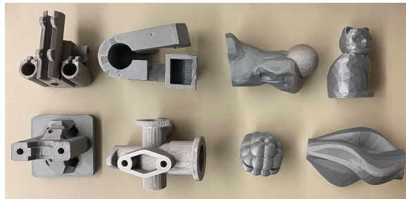
Figure 4.7: Physical objects for the grasp success prediction experiments using KUKA Robot with SCHUNK parallel-jaw gripper and RealSense D455 RGBD camera.
