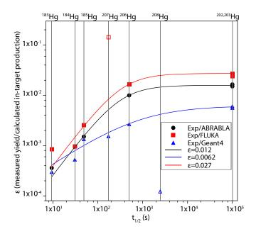
FIG. 3. Ionization and release efficiency ( $\varepsilon$ ) as a function of the half-life of mercury isotopes from a molten lead target. The results from ABRABLA, FLUKA, and GEANT4 simulations are compared. See text for details.
