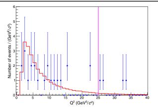
FIG. 3.  $Q^2$  distribution for data (blue dots) and MC simulation (red histogram). The area of MC distribution is normalized to that of data. The vertical (magenta) line indicates the selection requirement.
