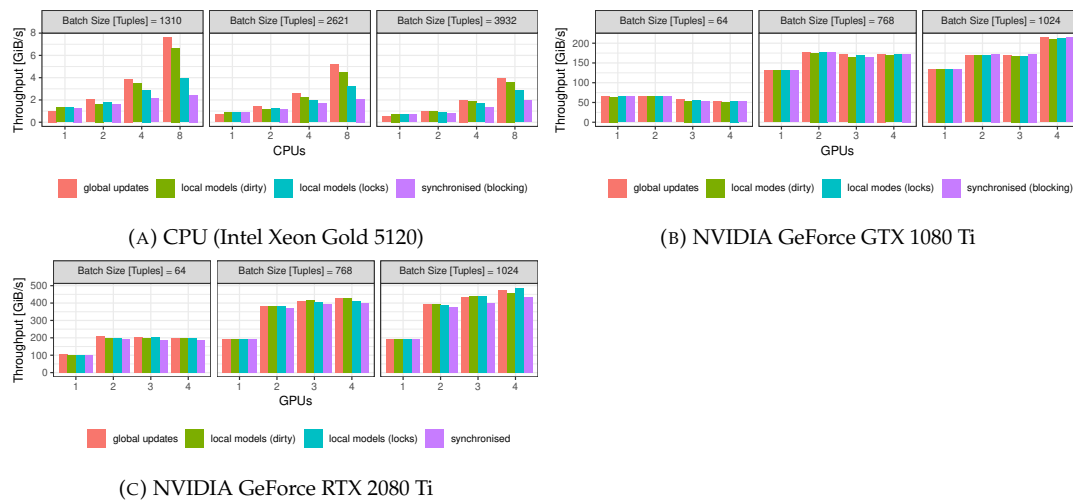
FIGURE 6.7: Scale-up for linear regression on (a) multiple CPUs, (b) multiple NVIDIA GeForce GTX 1080 Ti or (c) multiple NVIDIA GeForce GTX 2080 Ti.
