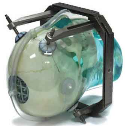
Inter-cranial Grid Phantom 335 Physical Control Points
