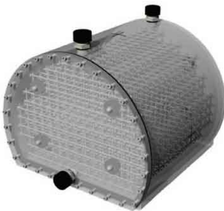
Large Field Grid Phantom 2152 Physical Control Points
