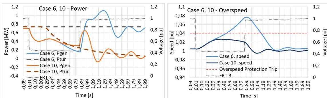
Figure 8: Comparison of power and overspeed on an asynchronous generator with fast valving (case 10) and without fast valving (case 6)
