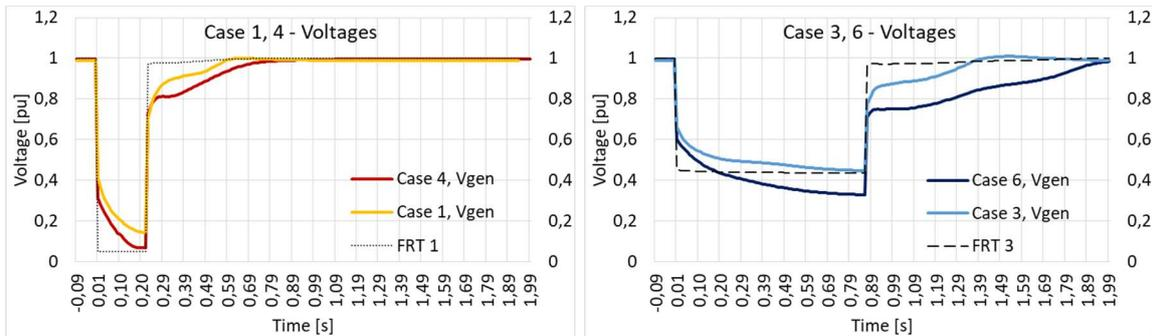
**Figure 4:** Comparison of voltage profiles between synchronous (case 1, 3) and asynchronous (case 4, 6) generators
