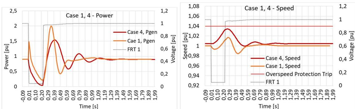
**Figure 5:** Comparison of power and overspeed between synchronous (case 1) and asynchronous (case 4) generators
