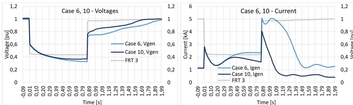
Figure 7: Comparison of voltage and current on an asynchronous generator with fast valving (case 10) and without fast valving (case 6)
