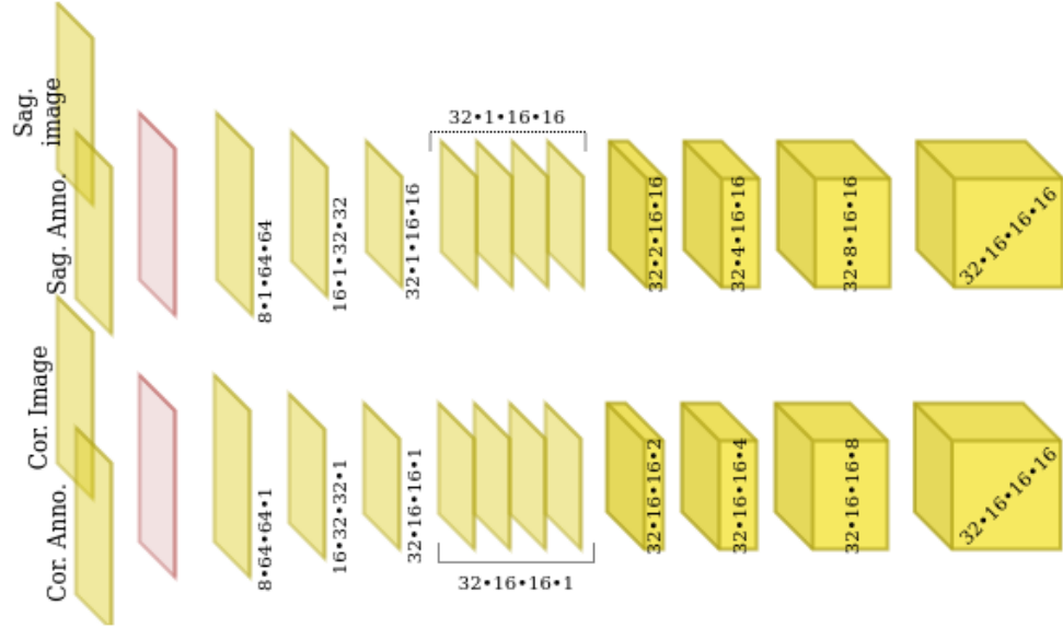
Figure A.4: Architecture of the orthogonal encoders, which employ anisotropic convolutions, with an anisotropy along the dimensions that need to be expanded. We use ‘squeeze and excitation’ blocks (depicted in red) to fuse the image features and annotation features.
