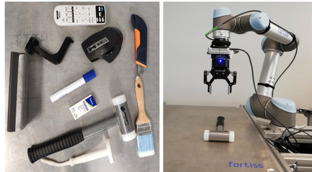
Fig. 7: Robot experiment setup with an UR5 robot arm
