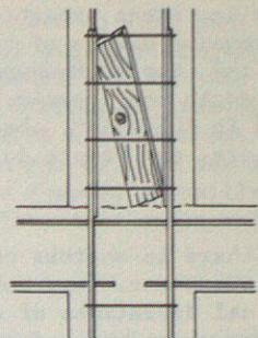
The third item (column with frozen concrete) is of a quite different nature. It is the material of the compression member itself that went a somewhat independent way. It was a cold winter and the heating wires inside the concrete did not work. Fig. 3.
