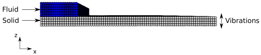
FIGURE III.22: Simulation set-up; liquid travelling on a vibrating solid plate.
