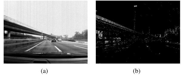
Fig. 6. Comparison of grayscale frame and event frame. (a) grayscale frame, (b) event frame.
