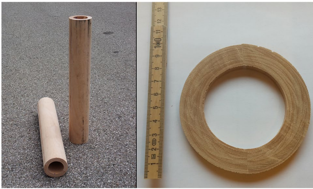
Fig. 1 Beech LVL hollow sections prototypes (left) and related cross section with 100 mm outer diameter and 18 mm wall thickness
