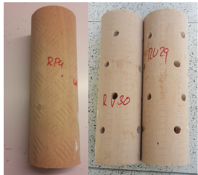
Fig. 6 LVL hollow cross section with veneer surface corrugations (left) and bore hole drillings (right)
