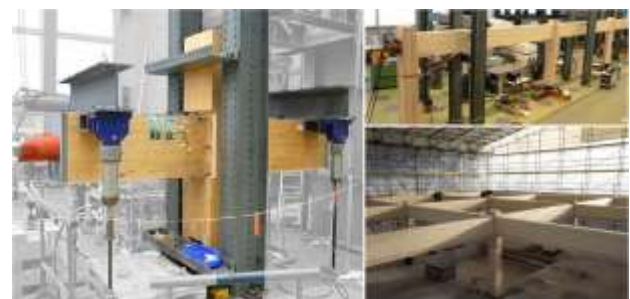
Figure 4: On the left glulam column-beam specimen; above on the right the entire three-spans frame and below the first floor of the ETH House of Natural Resources [32]
