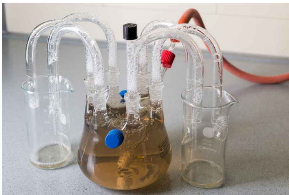
Figure 12: Self-made foam fractionation apparatus comprising six columns.
