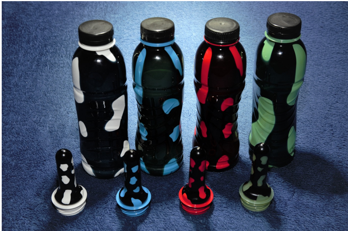
Figure 5: Developed silver doped preforms and bottles made of PET
