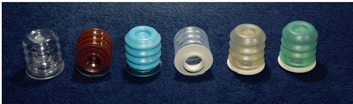
Figure 4: Developed bellows (from left): made of PET, made of PET and containing Ag-PURE, made of PET and containing silver phosphate glass, made of PP, made of PP and containing AgPURE, made of PP and containing silver phosphate glass
