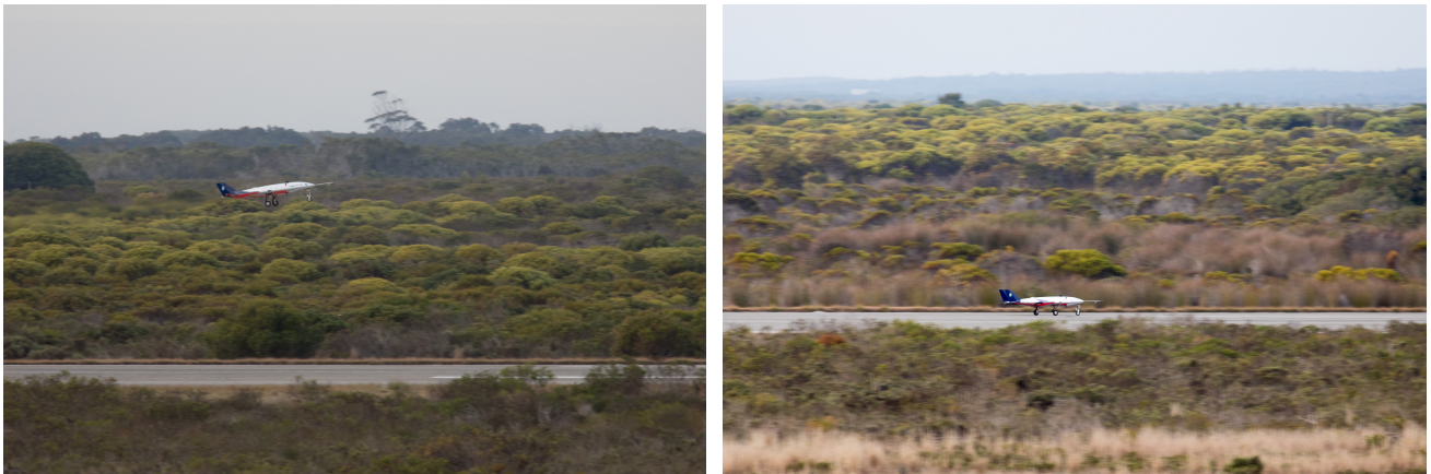
(a) Fully automatic final descent, shortly before touch-down (b) Automatic braking and centerline tracking, shortly after touch-down
