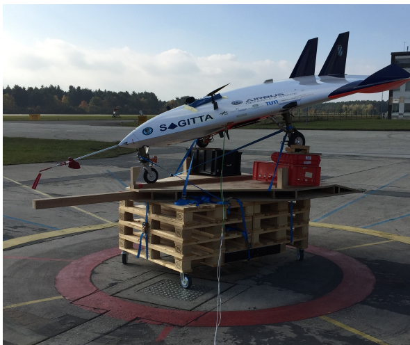
(b) Setup for magnetometer calibration
