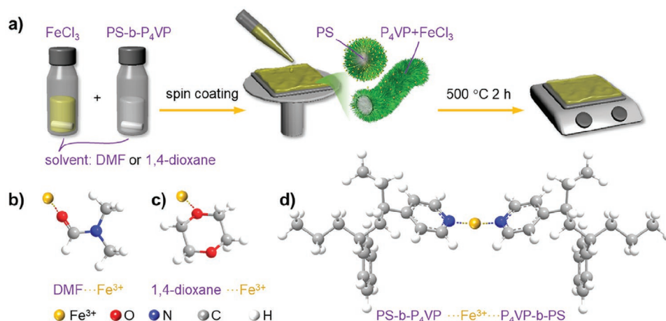
Figure 1. a) Preparation routine of PS- b -P 4 VP templated \alpha -Fe 2 O 3 thin films. Sketches of the complexation between FeCl 3 and solvent molecules: b) DMF...Fe 3+ complex and c) 1,4-dioxane...Fe 3+ complex. Complexation between d) FeCl 3 and PS- b -P 4 VP polymer template. Chlorine atoms are omitted for clarity of the presentation.
