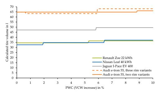
**Figure 6.** Interdependency between secondary volume change (SVC) of the wheel and the primary weight change (PWC).
