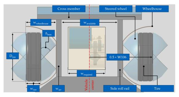
Figure 3. Overview of the relevant measures at the front end of the vehicle, based on Reference [3].
