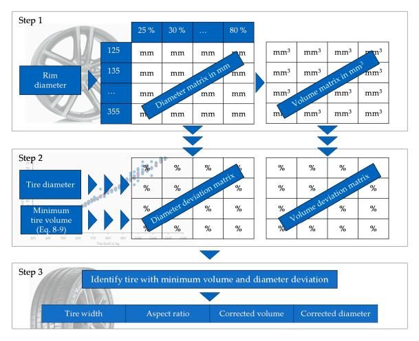
Figure 2. Overview of the correction method for the tire dimensions.
