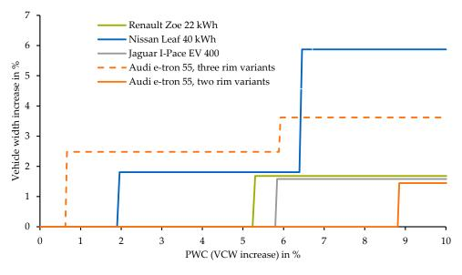
Figure 10. Interdependency between the vehicle width and the PWC.
