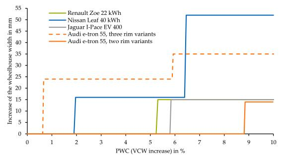
Figure 8. Interdependency between wheelhouse width and PWC.
