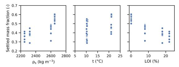
**Figure 4.** Settled mass fraction in the settling experiments with respect to  $\rho_s$ , t, and LOI; n = 33.
