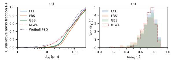
**Figure 1.** (a) Particle size distribution (PSD) of the analyzed samples and the fitted Weibull PSD used for the subsequent modeling, particle count: Eckenheimer Landstraße (ECL) n = 515,545; Frauensteinstraße (FRS) n = 593,302; Glauburgstraße (GBS) n = 540,036; MiW4 n = 501,254. (b) Mass fraction weighted histogram of  $\varphi_{\text{Riley}}$  of the analyzed samples, particle count: ECL n = 130,986; FRS n = 211,209; GBS n = 134,392; MiW4 n = 57,973.
