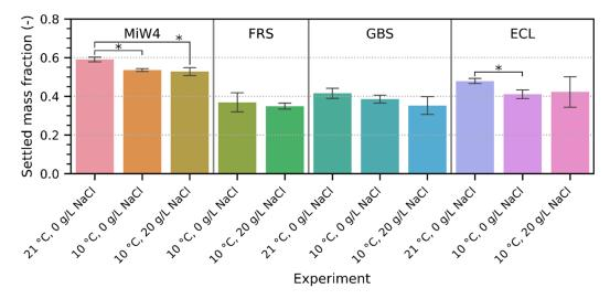
**Figure 3.** Settled mass fraction in the settling experiments with varying temperatures (21 and 10 °C) and NaCl concentrations (0 and 20 g/L); n = 3 for each experiment. The error bars indicate the standard deviation; the asterisks (\*) indicate statistically significant differences between two experiments (p < 0.05). Experiment FRS 21 °C 0 g/L NaCl was not conducted due to low sample quantity.
