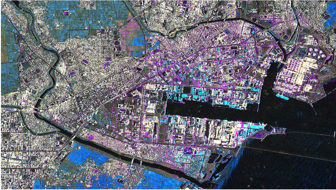
FIGURE 1.3: The TerraSAR-X image acquired on March 12, 2011 shows the impact of the tsunami on the port of Sendai, Japan ( DLR Portal, TanDEM-X - (August, 2020) "The port of Sendai after the tsunami" [Online] n.d. ). The blue colour indicates the flooded areas and the magenta colour highlights the damaged areas in the form of boulders.
