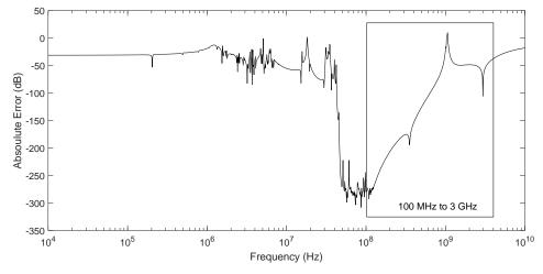
**Figure 14.** Absolute error of ROM generated using RNSZ of order N = 38 compared to original system frequency response of a spiral inductor (order n = 191). The mean absolute error is -129.98 dB from 100 MHz to 3 GHz frequencies.
