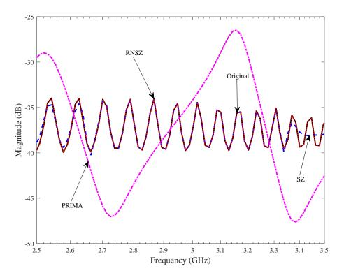
**Figure 9.** Magnitude response for the frequency of interest (2.5 GHz to 3.5 GHz) for an Intel Core i7-2920XM processor interconnect bus. The proposed method (RNSZ) closely matches the fine details of the original on-chip interconnect bus.
