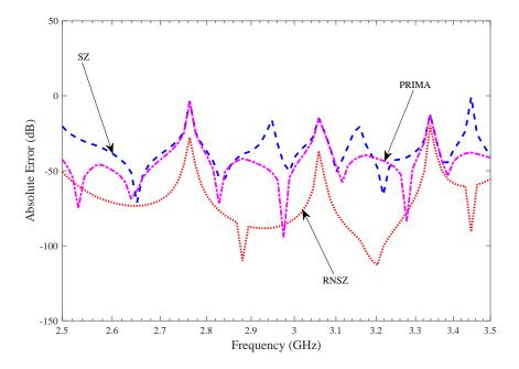
**Figure 5.** The absolute error plot shows minimum error for the RNSZ method. The calculated mean absolute error for the RLC network in the frequency of interest (2.5 GHz to 3.5 GHz) is -71.64 dB, -35.89 dB and -44.85 dB for RNSZ, SZ and PRIMA methods respectively.
