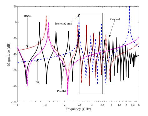
**Figure 3.** Frequency response of a on-chip RLC network with original system order of n = 79. The reduce models of using reduce norm spectral zero (RNSZ), PRIMA and spectral zeros (SZ) methods are of order N = 10. The reduce model generated by RNSZ closely matches the fine details of the original system compared to other techniques.
