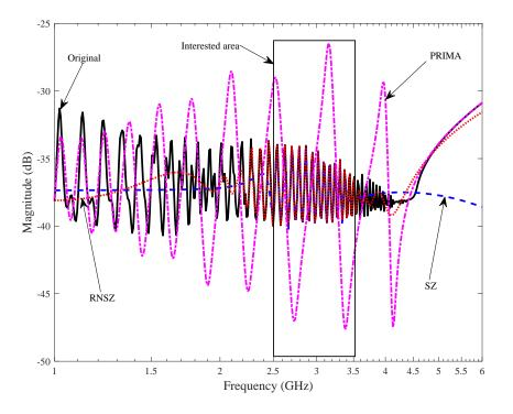
**Figure 8.** System frequency response of a interconnect bus with original system order n = 1076. The reduced order model (ROM) of order N = 100 for the other methods shows the response using RNSZ completely matches the original system.
