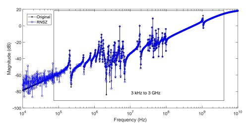
**Figure 19.** Original system frequency response of a spiral inductor (order n = 191) compared with a ROM generated using a high order (N = 186) RNSZ method covering 3 kHz to 3 GHz frequencies.
