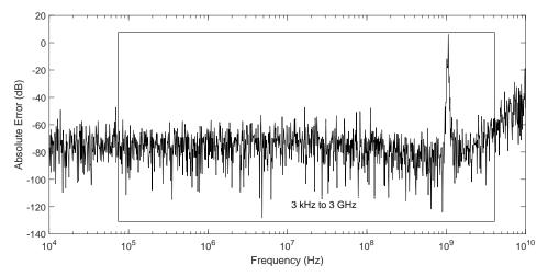
**Figure 20.** Absolute error of ROM generated using RNSZ of order N = 186 compared to original system frequency response of a spiral inductor (order n = 191). The mean absolute error is -76.29 dB from 3 kHz to 3 GHz frequencies.
