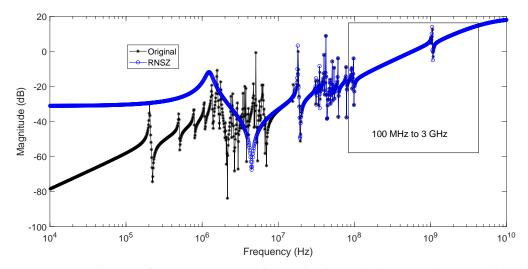
**Figure 13.** Original system frequency response of a spiral inductor (order n = 191) compared with a ROM generated using RNSZ of order N = 38 covering 100 MHz to 3 GHz frequencies.
