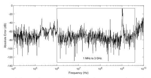
**Figure 18.** Absolute error of ROM generated using RNSZ of order N = 180 compared to original system frequency response of a spiral inductor (order n = 191). The mean absolute error is -73.98 dB from 1 MHz to 3 GHz frequencies.
