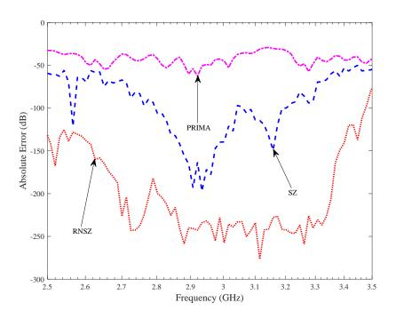
**Figure 10.** The absolute error plot shows minimum error for the RNSZ method. The calculated mean absolute error for the interconnect bus example in the frequency of interest is -180.52 dB, -112.93 dB and -42.61 dB for RNSZ, interpolation by SZ and PRIMA methods respectively.
