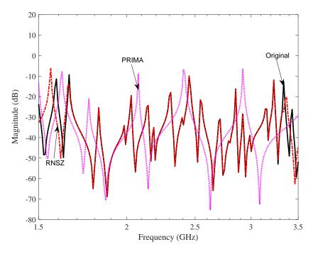
**Figure 11.** System frequency response of a spiral inductor with original system order of n = 1008. The selected large span of frequency now cover over 2 GHz of frequency range, i.e., from 1.5 GHz to 3.5 GHz. A minimum ROM of order N = 50 is required by RNSZ method to match the response. However, with similar ROM (N = 50), the PRIMA method missed out most of the response and peaks of the original system.
