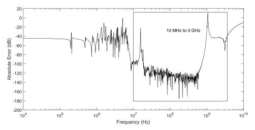
**Figure 16.** Absolute error of ROM generated using RNSZ of order N = 50 compared to original system frequency response of a spiral inductor (order n = 191). The mean absolute error is -100.97 dB from 10 MHz to 3 GHz frequencies.
