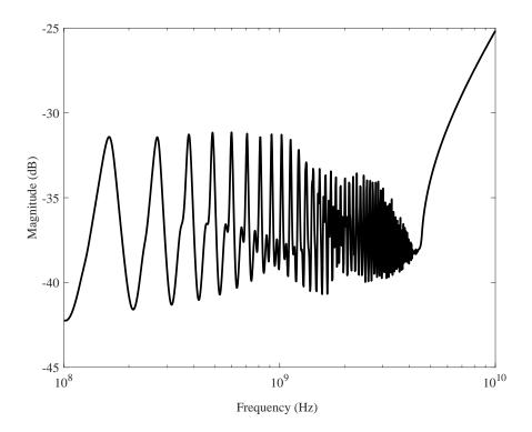
Figure 7. Original system frequency response generated by a interconnect bus of order n = 1076.
