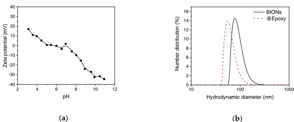
**Figure 2.** (a) Zeta potential of BIONs at various pH-values titrated from pH 3 to pH 11 with sodium hydroxide (0.1 M). (b) Size distribution of coated @Epoxy and uncoated BIONs, determined by dynamic light scattering (DLS) at pH 10.
