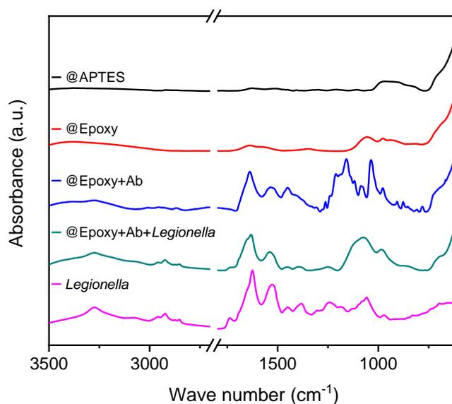
**Figure 4.** Attenuated total reflection infrared (ATR IR)-spectra of APTES-coated BIONs, @Epoxy nanoparticles with and without immobilized antibodies. The spectra of particles with immobilized antibodies is shown before and after coupling with *Legionella* and the spectrum of *Legionella* is shown.
