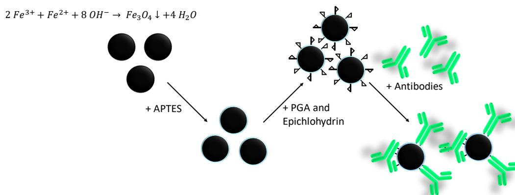
**Scheme 1.** Schematic illustration of the iron oxide synthesis, APTES coating, polyglutaraldehyde (PGA) functionalization, epichlorhydrin activation, and antibody coupling.
