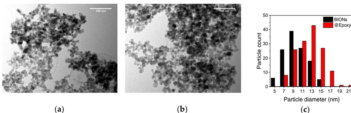
**Figure 1.** Transmission electron microscopy (TEM)-microphotography of bare iron oxide nanoparticles (BIONs) (a) and of @Epoxy particles (b). Frequency distribution of pure BIONs and PGA-coated SPIONs with various particle diameters, measured by TEM (c).
