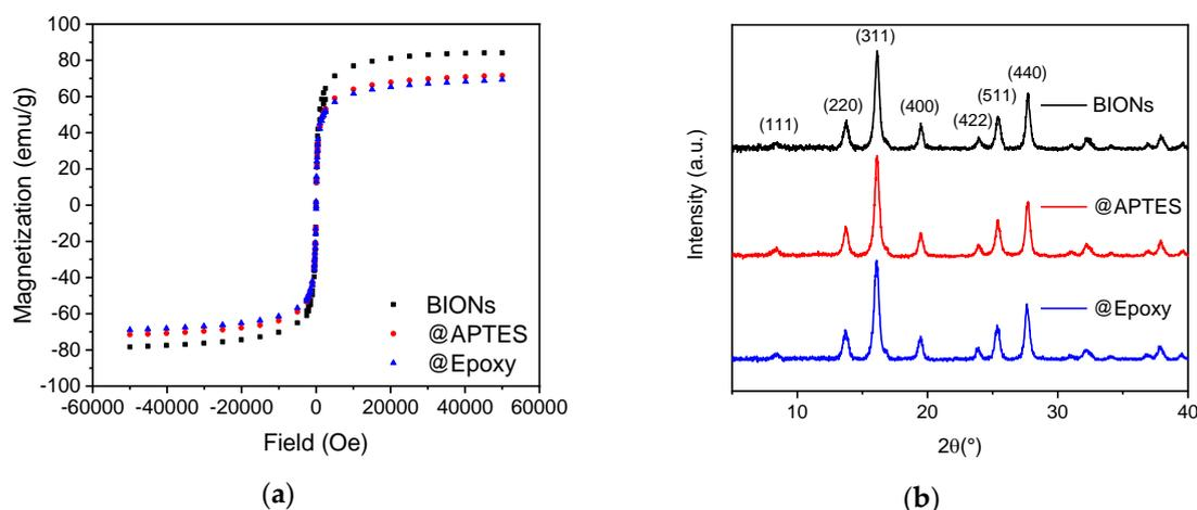
**Figure 3.** (a) SQUID-analysis of pure and coated BIONs at 300 K. (b) Powder X-ray diffractograms of different nanoparticles.
