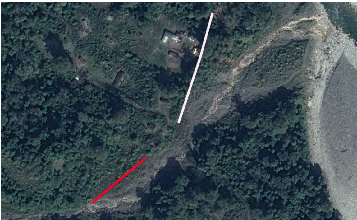
Figure 13.3: The penstock location as per the original design (red), and the new location (white).[93].
