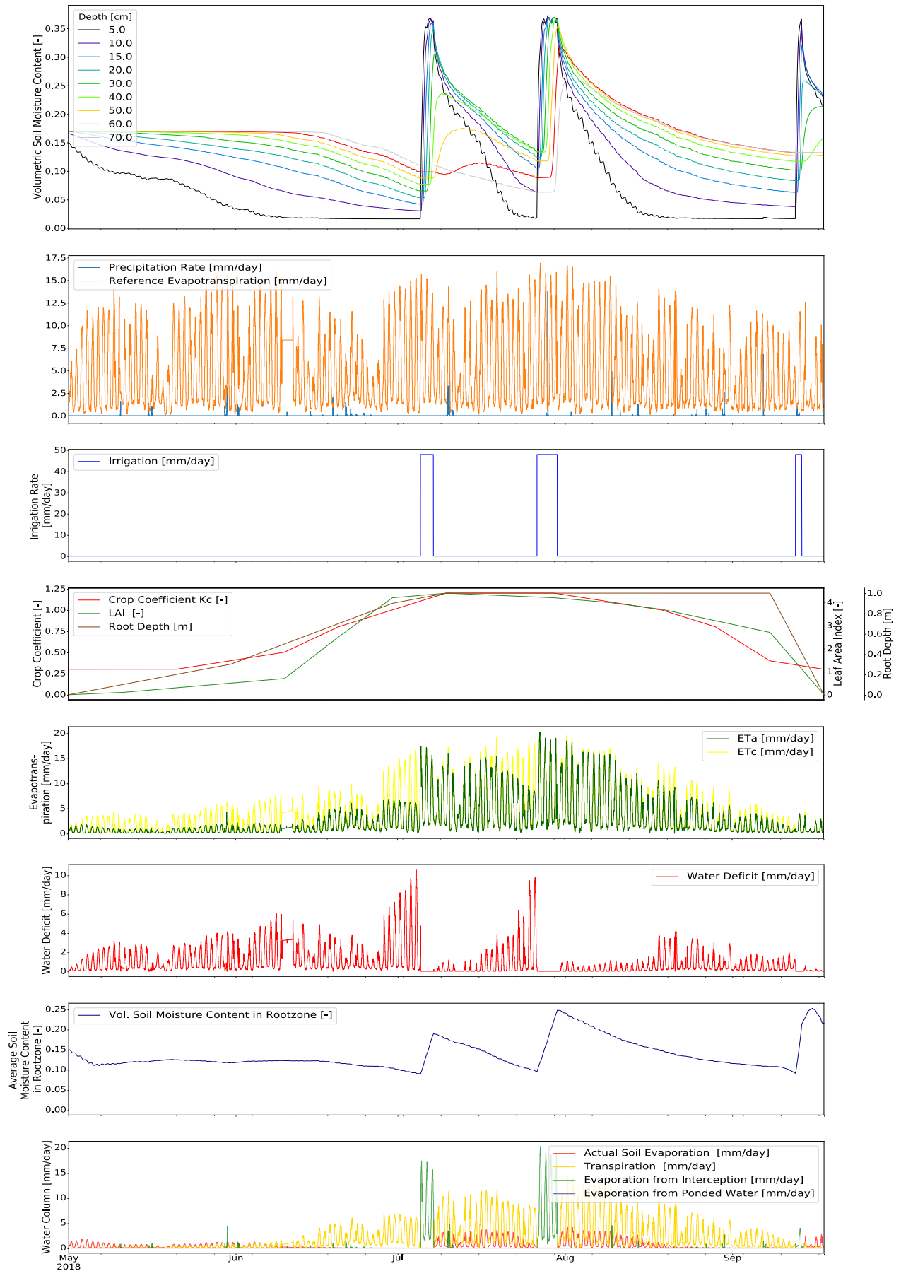
Figure 29: Overview optimization with MIKE SHE - result of a seasonal simulation for the dry year 2018.
