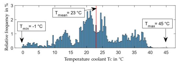
Figure 6. Machine winding overhang temperature for the NEmo.
