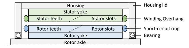
Figure 7. Individual components of the induction machine (IM) in a radial section.
