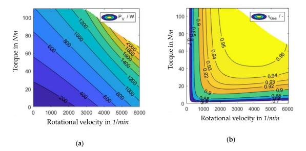
Figure 1. (a) Power dissipation diagram and (b) efficiency diagram of an electric machine [7].
