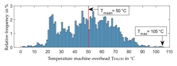
Figure 5. Machine winding overhang temperature for the NEmo.
