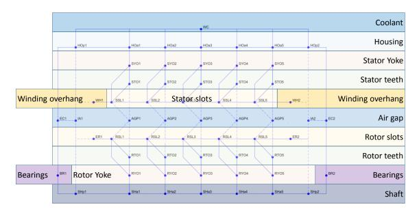
machine in electric vehicles because it allows the power and torque density of the electric machine to be increased [28]. The overall thermal network implemented in this article is illustrated in Figure 8.
