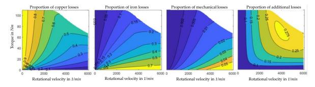
Figure 2. Proportion of different loss types in the efficiency diagram of the machine.
