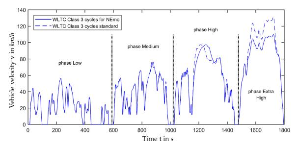
**Figure 4.** Speed curve of the standard and worldwide harmonized light vehicles test cycle (WLTC) driving cycle adapted for the NEmo [20] (p.22).
