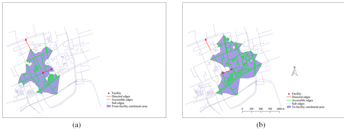
Figure 9. The from-facility (a) and to-facility (b) catchment area of a point facility based on a directed road network.
