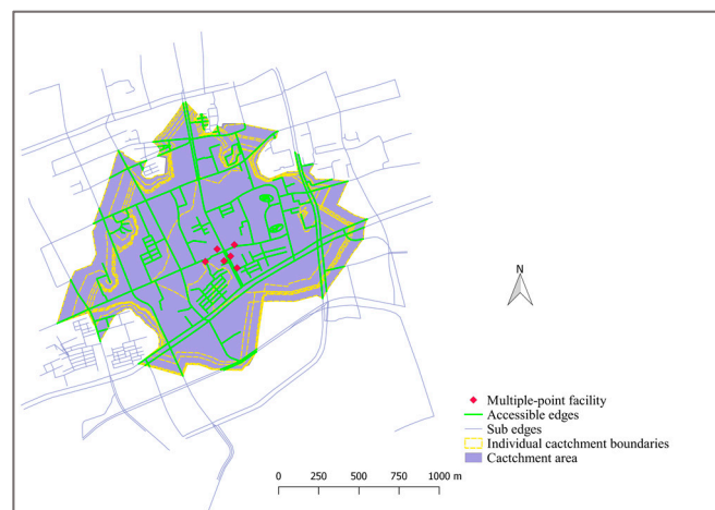
Figure 10. The catchment area of a multiple-point facility based on an undirected road network.
