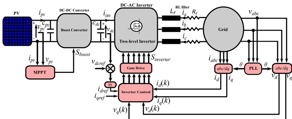
Figure 1. Block diagram of the PV system under study.
