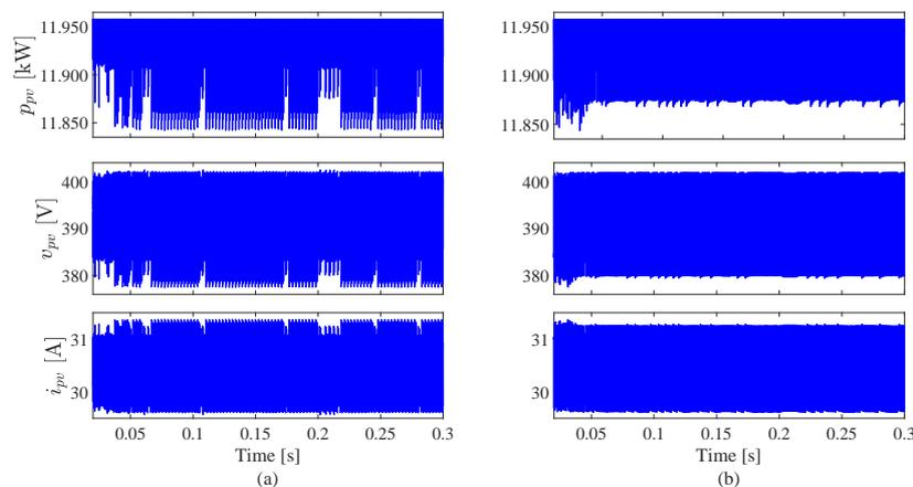
**Figure 17.** MPPT performance at constant atmospheric conditions with: (a) conventional MPPT and (b) direct switching technique.
