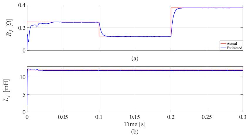
**Figure 20.** Estimated and actual values of the filter parameters with different step changes in the filter resistance: (a) filter resistance and (b) filter inductance.
