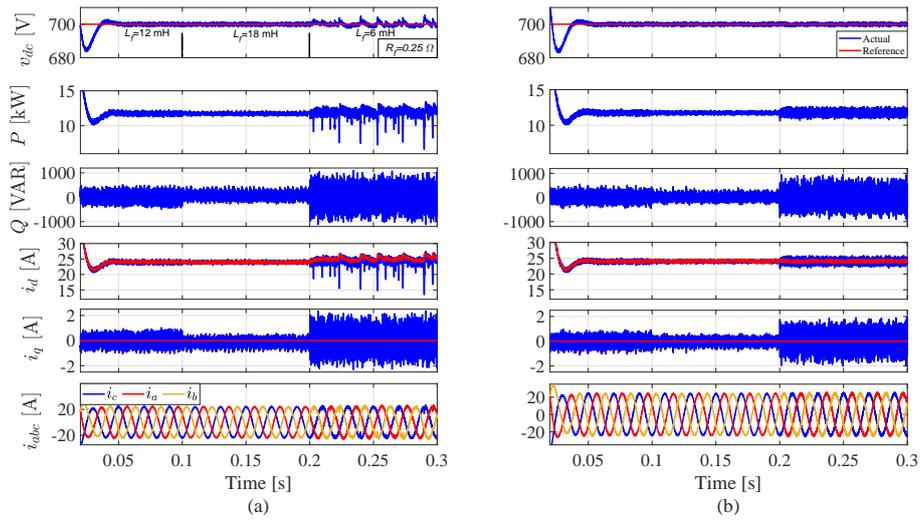
**Figure 21.** Simulation results at different step changes of the filter inductance (from top): DC-link voltage, grid injected active power, reactive power, d-axis current, q-axis current and abc currents for: (a) conventional FCS-MPC and (b) proposed FCS-MPC with EKF.
