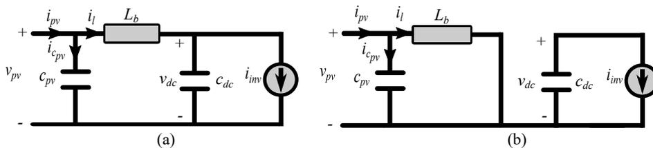
Figure 7. Equivalent circuit of the boost converter when: (a) Switch is off, and (b) switch is on.
