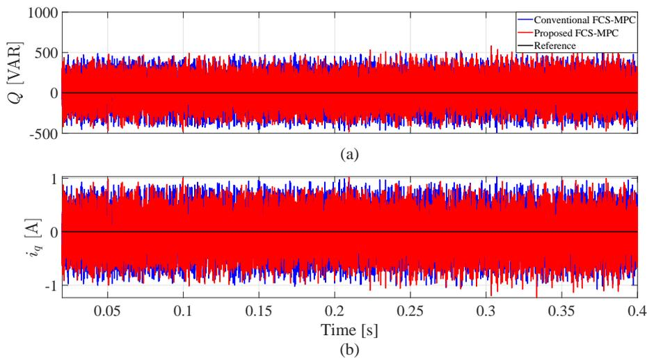
**Figure 15.** Comparison between the proposed and the conventional FCS-MPC at different radiation conditions: (a) reactive power and (b) q-axis current.
