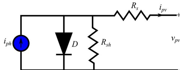
Figure 2. Single diode model of the PV module.
