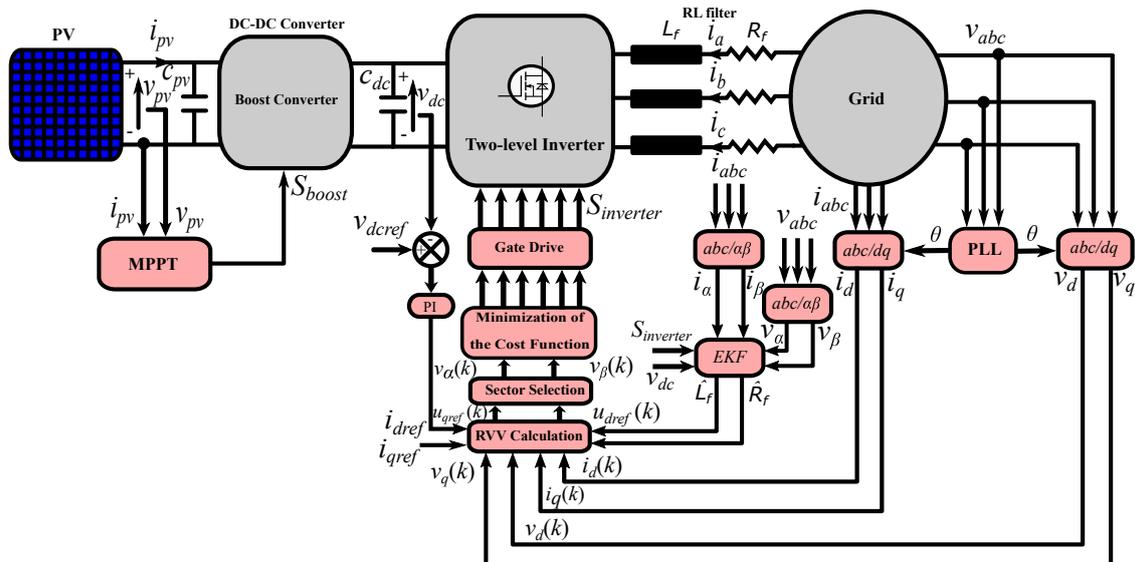
Figure 11. Proposed FCS-MPC of the PV grid connected system.
