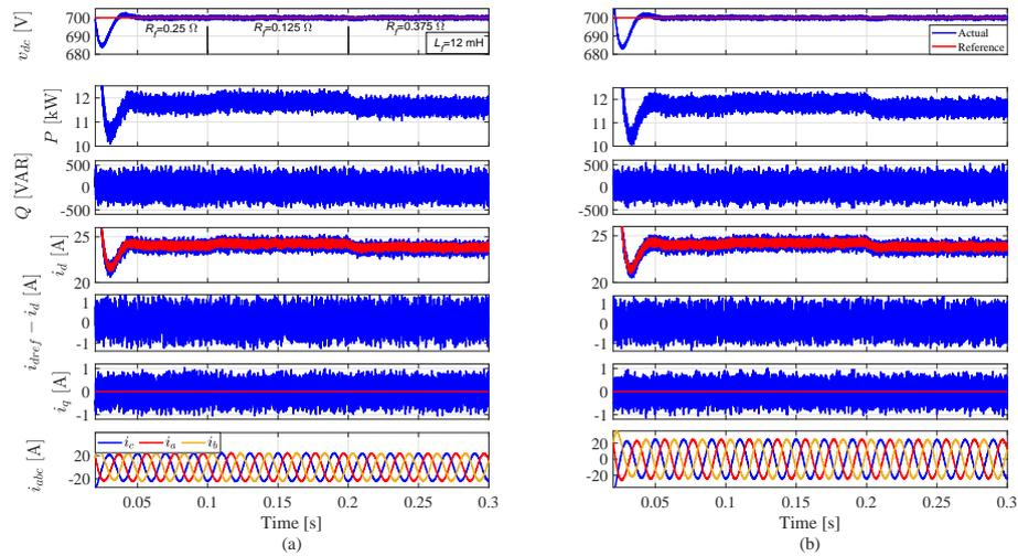
**Figure 18.** Simulation results at different step changes of the filter resistance (from top): DC-link voltage, grid injected active power, reactive power, d-axis current, error in d-axis current with respect to the reference, q-axis current and abc currents for: (a) conventional FCS-MPC and (b) proposed FCS-MPC with EKF.
