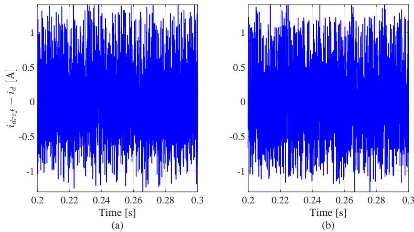
**Figure 19.** Error between d-axis current and its reference for: (a) conventional FCS-MPC and (b) proposed FCS-MPC with EKF.
