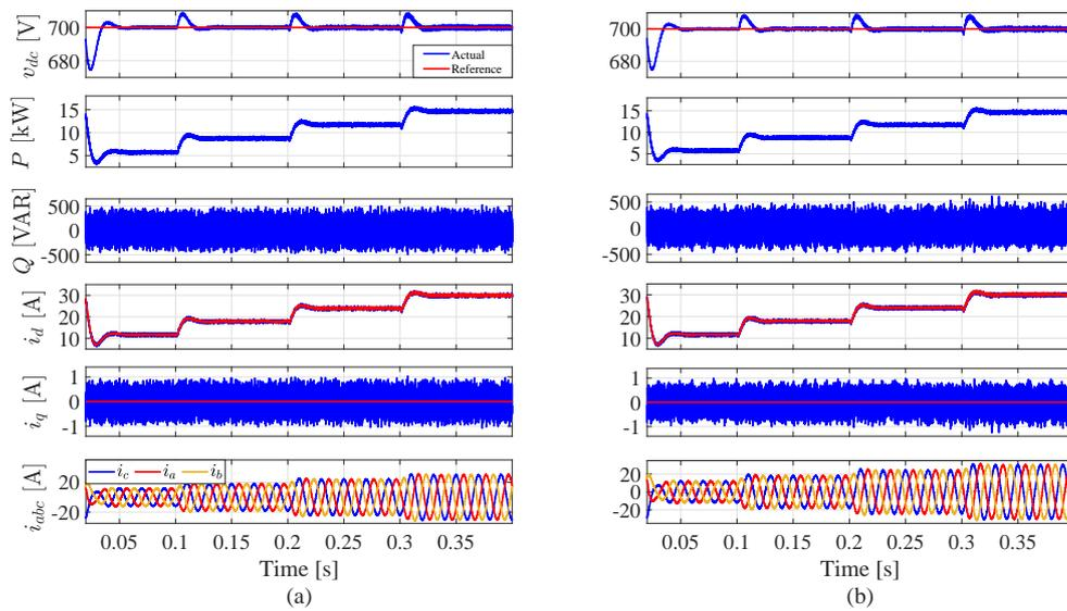
**Figure 14.** Simulation results at different step changes of radiation of the grid connected PV inverter (from top): DC-link voltage, grid-injected active power, reactive power, d-axis current, q-axis current and abc currents for: (a) conventional FCS-MPC and (b) proposed FCS-MPC with EKF.
