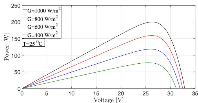
Figure 3. P–V characteristics of the PV module under different radiation conditions and constant temperature.
