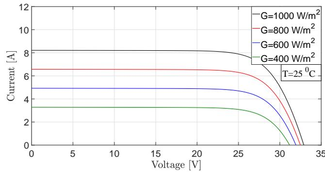
Figure 5. I–V characteristics of the PV module under different radiation conditions and constant temperature.
