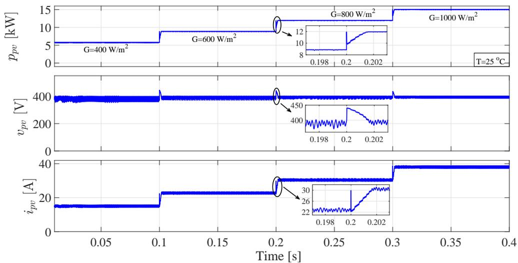
Figure 12. Performance of the conventional MPPT using FCS-MPC.
