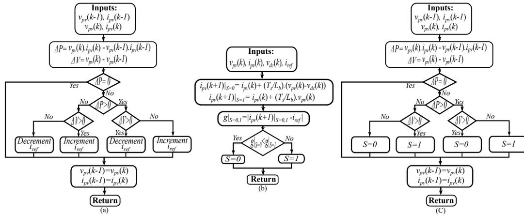
Figure 8. (a) P&O scheme to generate the reference current for FCS-MPC. (b) FCS-MPC procedure to generate the switch state. (c) The proposed direct switching MPPT technique.
