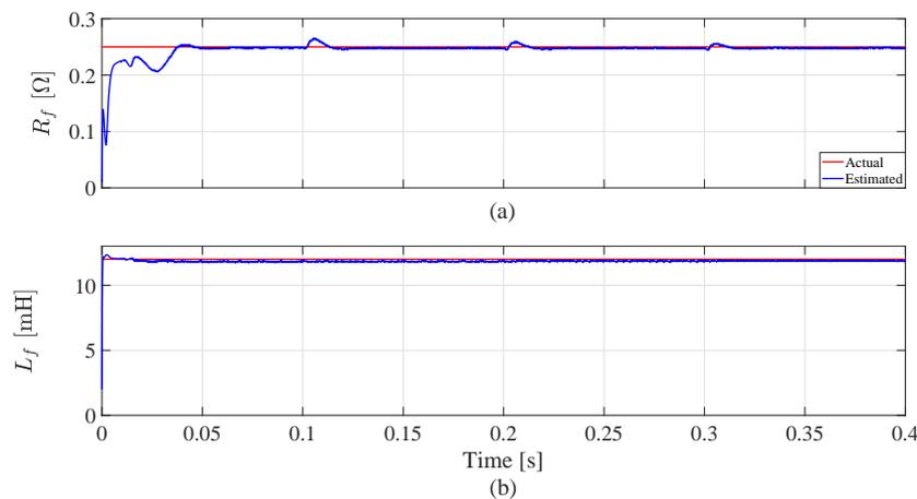
**Figure 16.** Estimated and actual values of the filter parameters with different radiation conditions: (a) filter resistance and (b) filter inductance.
