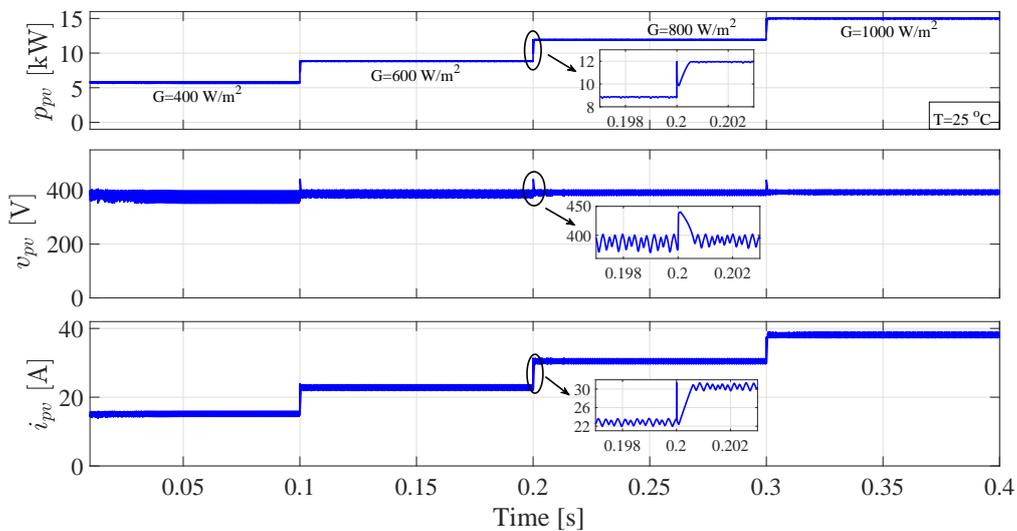
Figure 13. Performance of the proposed direct switching MPPT.
