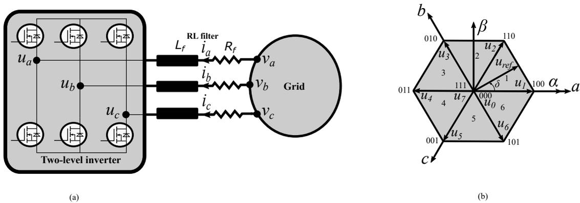
Figure 9. (a) Two-level voltage source inverter with grid connection. (b) Switching actions and voltage vectors of the inverter.
