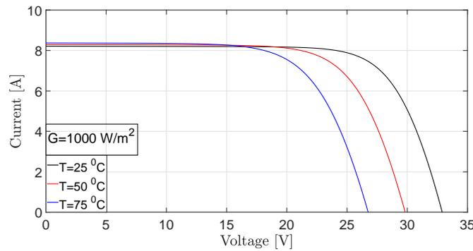
Figure 6. I–V characteristics of the PV module under different temperature conditions and constant radiation.
