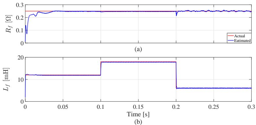
**Figure 23.** Estimated and actual values of the filter parameters with different step changes in the filter inductance: (a) filter resistance and (b) filter inductance.
