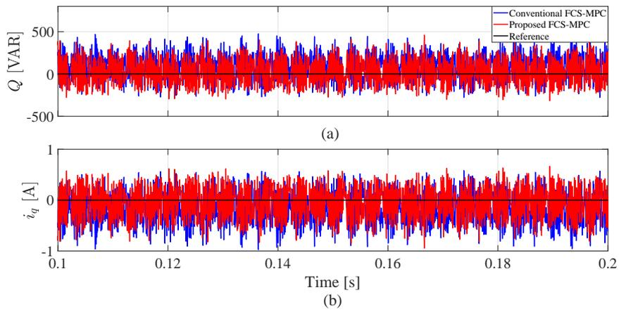
**Figure 22.** Comparison between the proposed and the conventional FCS-MPC: (a) reactive power and (b) q-axis current.
