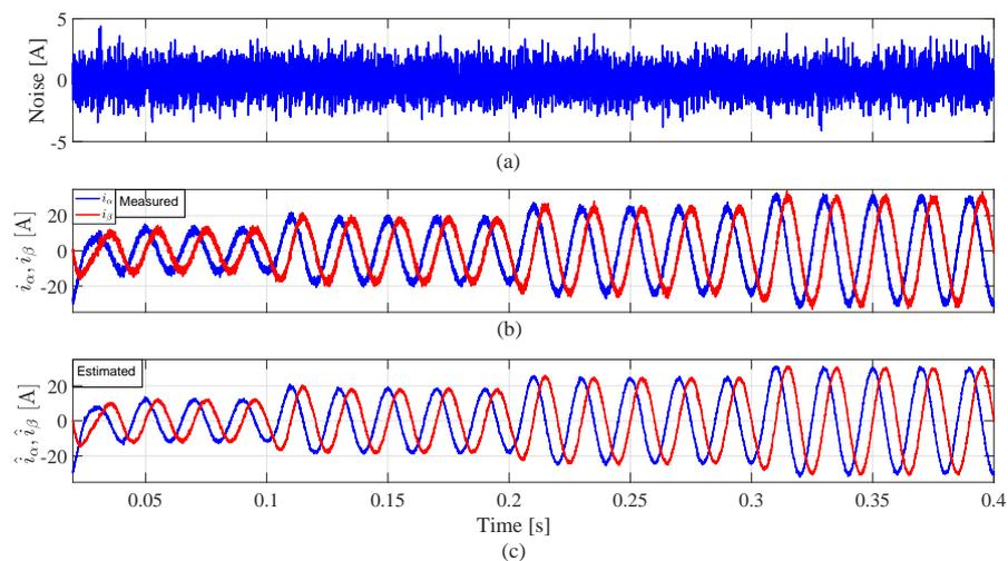
**Figure 24.** Estimated and noisy  $\alpha\beta$  currents: (a) added noise, (b) the noisy currents and (c) estimated (filtered) currents.
