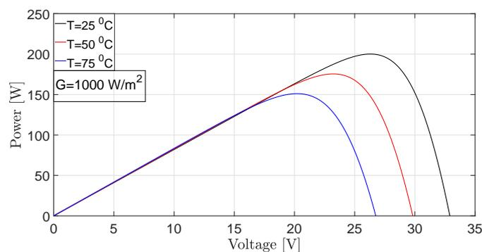
Figure 4. P–V characteristics of the PV module under different temperature conditions and constant radiation.
