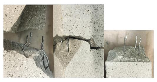
Figure 18. Fracture surface depending on the bond behavior.
