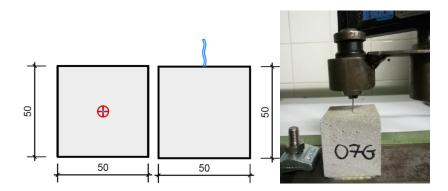
Figure 5. Pull-out tests of the wire fibers: schematic overview (left) and sample (right).
