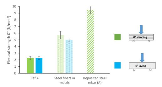
**Figure 6.** Flexural strength of lightweight mortar specimen: reference, with micro steelfibers and with deposited steel rebar (cut out 0° to printing direction, tested standing (**green**) and laying (**blue**).
