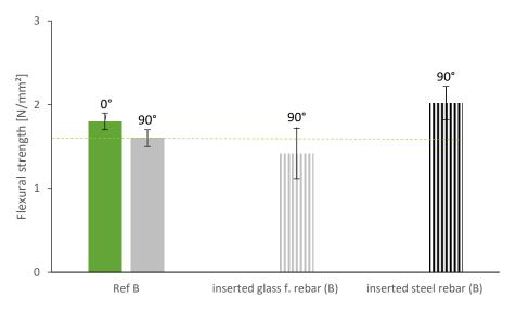
Figure 12. Flexural strength of specimen with vertically inserted rebars.
