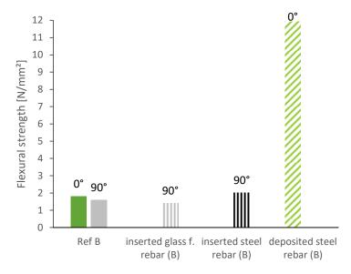
**Figure 14.** Flexural strength depending on the bond between the rebar (steel/glass fiber) and the mortar in comparison to flexural strength of the reference mixture.
