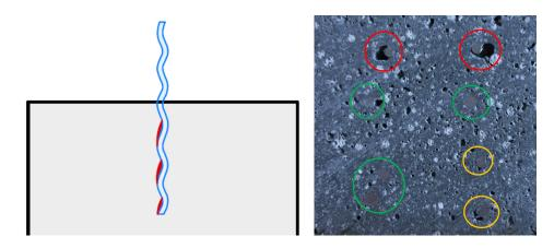
**Figure 17.** Schematical cavity formation around the vertically inserted fibers (**left**). Different quality of bond between fibers and mortar (**right**—red: bad, yellow: satisfactory, green: good bond behavior).
