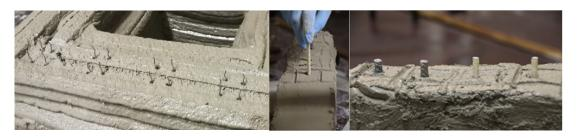
Figure 3. Vertical insertion of reinforcement: wire fibers (left), rebars (middle and right).
