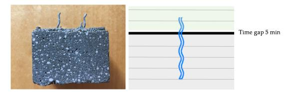
**Figure 10.** Specimen with vertically inserted fiber reinforcement over cold joints (**left**) and schematically area of fracture (**right**).
