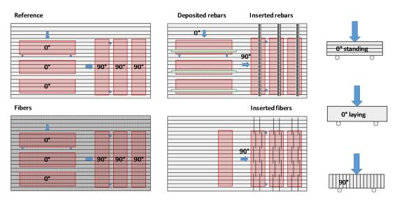
Figure 4. Schema of test prism cut out of 3D-printed element and test directions for flexural strength.
