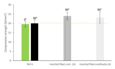
Figure 11. Compressive strength of specimen with vertically inserted fiber reinforcement.
