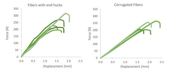
Figure 13. Fiber pullout tests of specimen with vertical fiber reinforcement.
