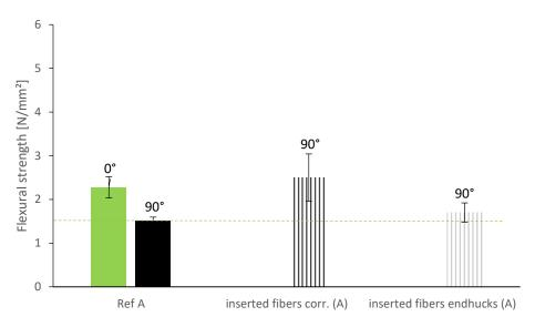
Figure 9. Flexural strength of specimen with vertically inserted fiber reinforcement.
