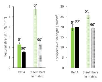
**Figure 7.** Flexural and compressive strength of specimen without and with micro steelfibers (cut out  $0^{\circ}/90^{\circ}$  to printing direction).
