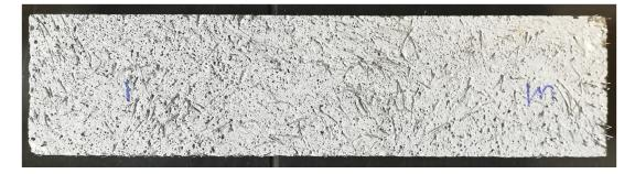
Figure 8. Micro steelfiber orientation in a prism sawn out from a 3D-printed object (side view).
