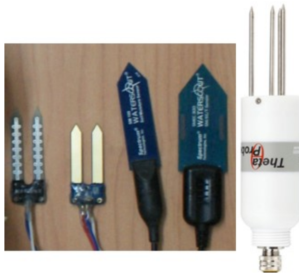
Figure 1. The four soil moisture sensors investigated in the study; from left to right (in the order of ascending cost): YL69, YL100, SM100, and SMEC300. The rightmost sensor is the secondary standard sensor, ThetaProbe.
