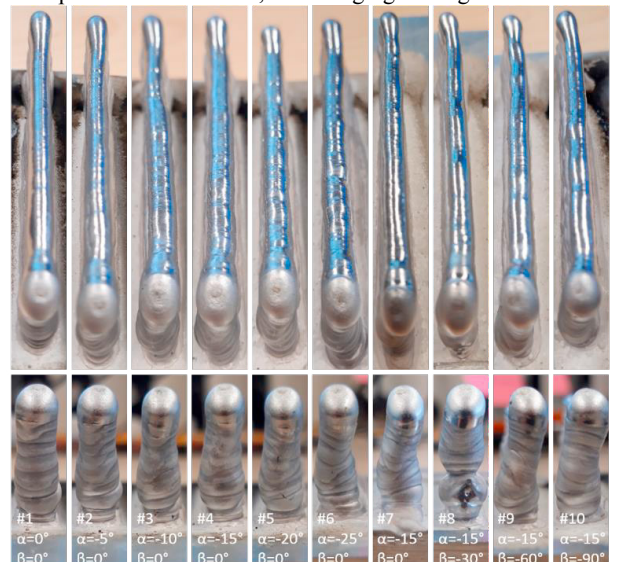
Fig. 4. Influence of different lead angles ( 0^\circ , 5^\circ , 10^\circ , 15^\circ , 20^\circ , 25^\circ ) on the wall geometry (height and width), inclination of the wall and surface smoothness
