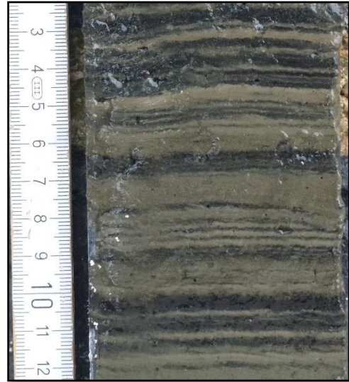
Figure 1.6: Section of the varved sediment core from the Lake Enge-ratsgundsee. Dark organic layers form during summer, bright inorganic in winter or after heavy precipitation events.
