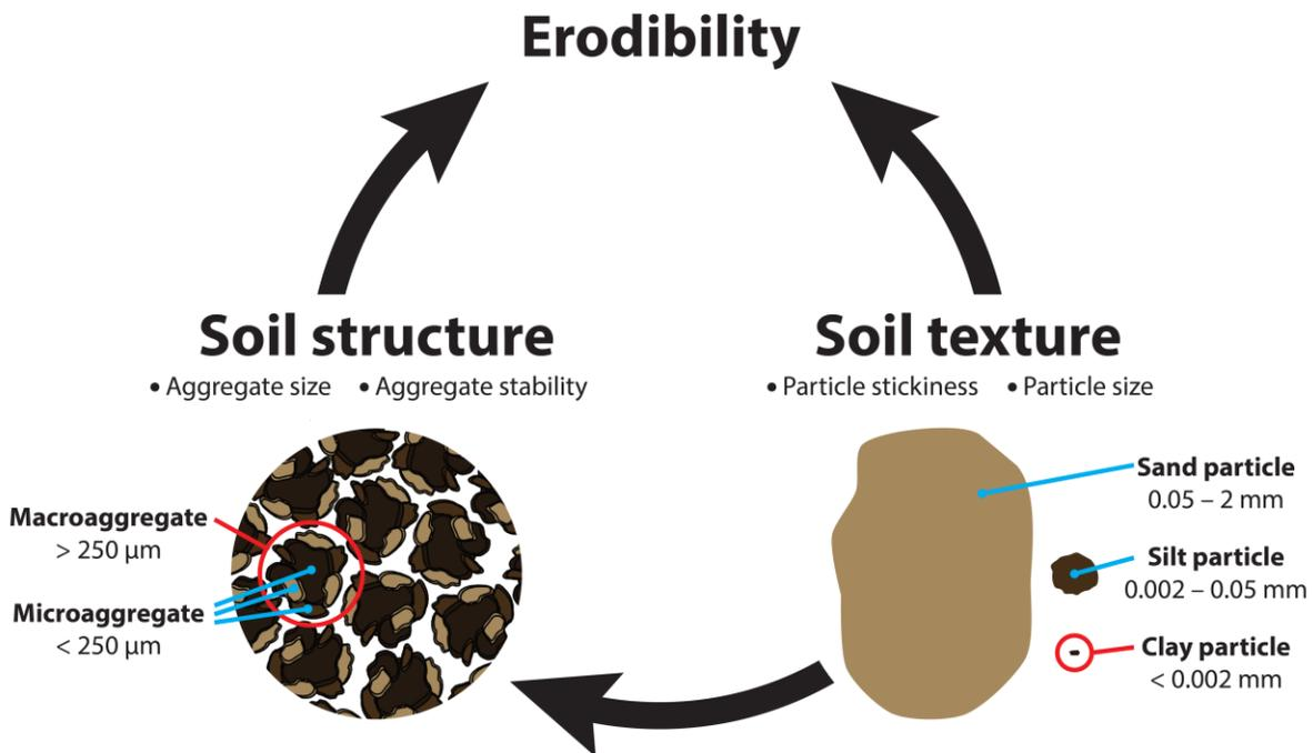
**Figure 1.** Soil parameters and their most important aspects influencing erodibility. The dependencies between those parameters and erodibility are marked with directional arrows.
