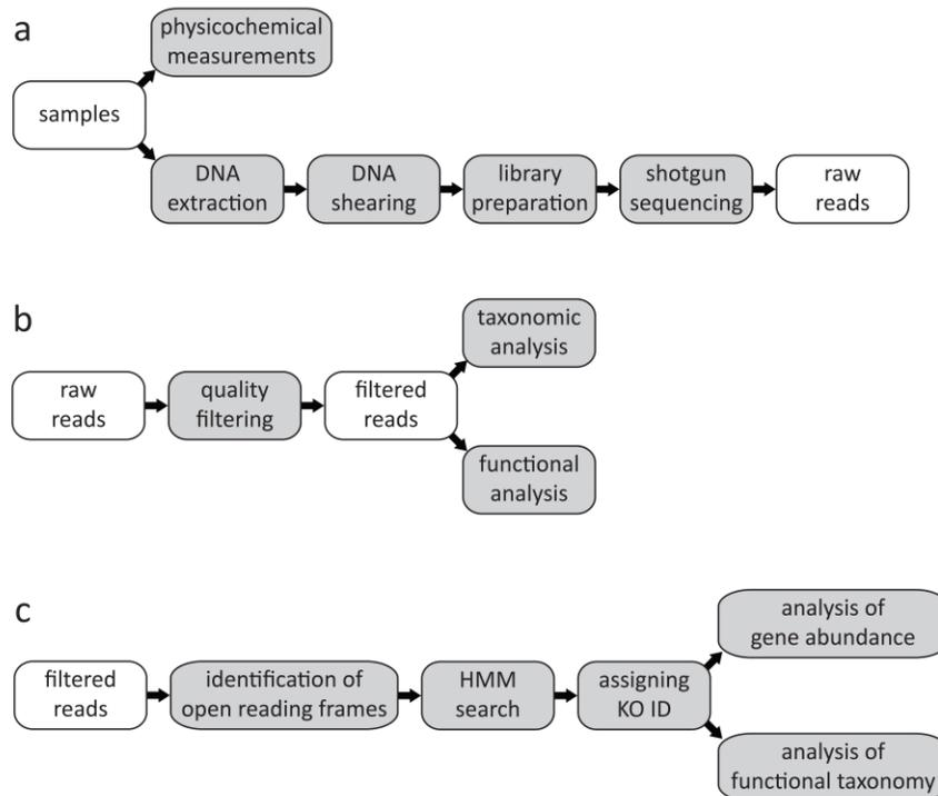
**Figure 8.** Schemes demonstrating the workflows of a) sample processing, b) general bioinformatical processing of sequencing data and c) functional analysis of genes specific for EPS and LPS biosynthesis.
