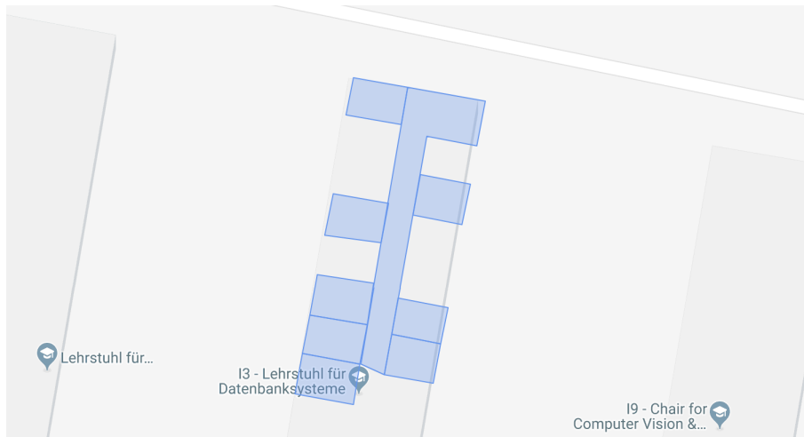
Figure (3.8) The localization area segmented into polygons based on topology, visualized in Google Maps. The gaps in the map are restricted area.
