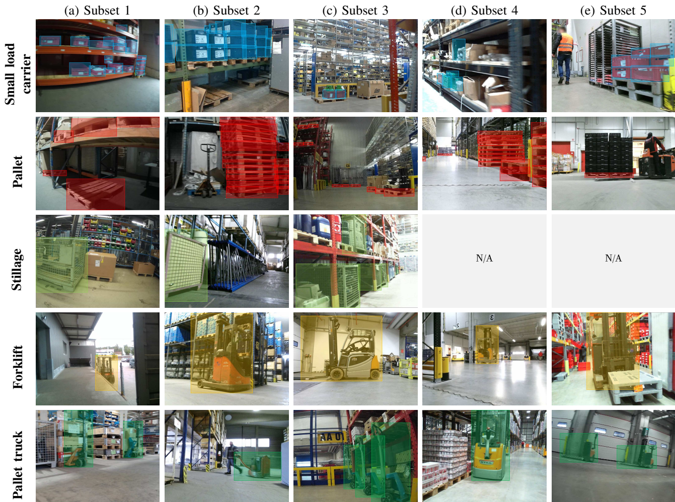
Fig. 3. LOCO sample images. The figure shows different object categories labeled throughout different subsets. For illustration purposes, only labels of specified classes are shown. Note the object difference within classes (e.g. pallet truck), image quality due to different cameras, and the contextual difference within subsets. In addition, subset four and five do not contain stillage instances, as they are not common within distribution centers.
