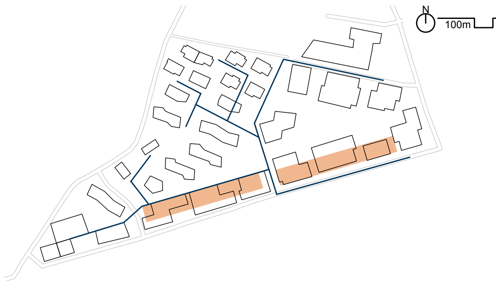
Figure 2-6: Topology of the Anergy Network in Rotkreuz, Switzerland (Vetterli et al. 2017; Open Street Map Foundation 2019)
