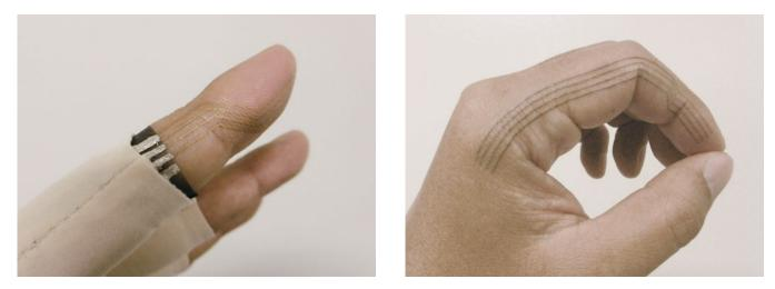
2 | Ultrathin nanomesh sensor directly applied on the finger of a human participant. These sensors are designed to measure a biological information (pressure, temperature, strain, etc).
