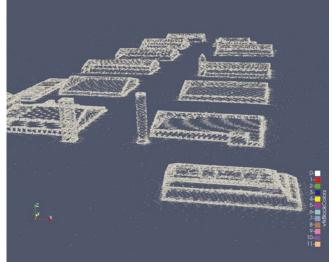
2 | CAD mesh model of Oktoberfest for CFD simulation.
