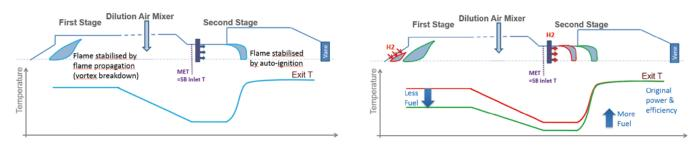
1 | Schematic of sequential combustion with flame positions for natural gas (left) and hydrogen (right). Copyright Ansaldo Energia.
