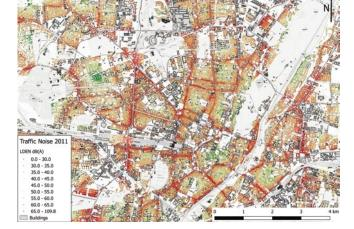
2 | Simulated noise caused by traffic in Munich
