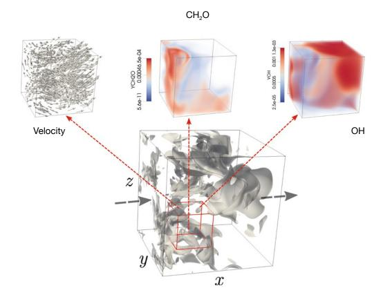
2 | Bayesian data assimilation enables the spatiotemporal prediction of seemingly random ignition spots in a turbulent reacting flow direct numerical simulation [5].
