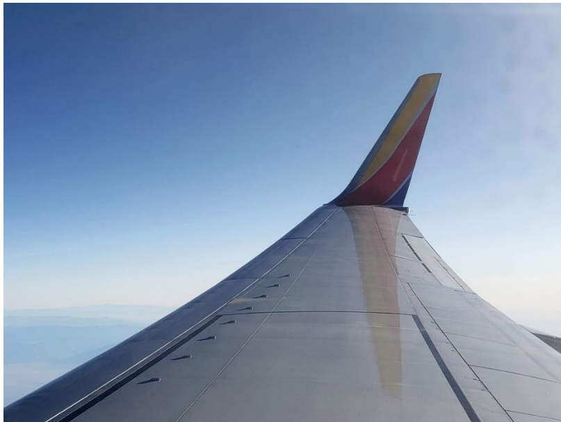
Figure 5-5. Wing of Boeing 737-700 narrow-body airliner with winglet.
