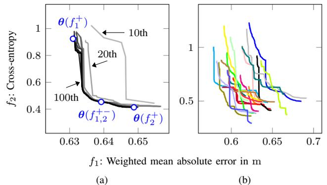
Fig. 4. (a) Evolution of frontiers  $\mathcal{F}_1$  in the 10th, 20th, ..., 100th generation of the GA from an experiment in gray color with increasing darkness for later generations. The blue circles represent the positions of 3 selected parameter sets in the objective function space according to different criteria. (b) Frontiers  $\mathcal{F}_1$  in their 100th generation of the GA from all 20 experiments.
