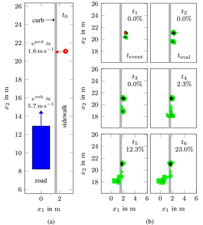
Fig. 6. A stopping trajectory in [27] with the same annotations as in Fig. 5. Although the recording stops after  $t_1$  and the ground truth position therefore only exists at  $t_1$  in part (b), we regard our prediction as a true negative w.r.t. crossing in front of the vehicle based on the labeling of this recording and the predicted occupancy on the road at  $t_2$  ( $t_{\text{eval}}$ ) of 0.0% probability.
