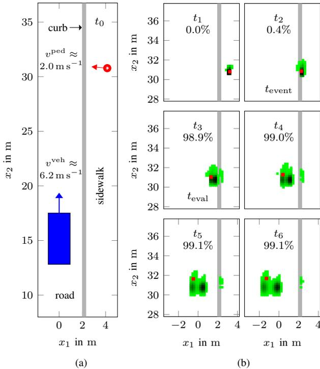
Fig. 5. A crossing trajectory in [27]. (a) The initial positions and velocities of the pedestrian (red circle) and the vehicle (blue rectangle) at  $t_0$ . (b) The green cells illustrate the predicted occupancies using  $\text{MC-}\theta(f_{1,2}^{+-})$  in different time steps (the darker the color, the higher the probability); the red squares represent the ground truth positions at different points in time; the numbers in each box are the summed probability of green cells on the road.
