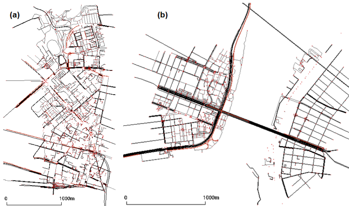
Figure 3 Microscopic traffic flow simulations networks in SUMO for the locations of (a) Munich, Germany, and, (b) NYC, USA
